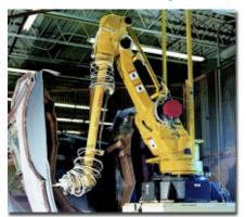
Precision robotic waterjet cutting is used to ensure part to part trimming accuracy.
