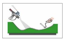
Similar to hand lay-up in simplicity, spray-up offers greater shape complexity and faster production. It too uses a low-cost open mold (one finished part surface), room temperature curing resin, and is suited for producing large FRP/Composite parts such as tub/shower units and vent hoods in low to moderate quantities. Cure is usually at room temperature, but can be accelerated by application of moderate heat.
