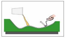
The simplest and oldest of the fabrication processes for FRP/ Composites, hand lay-up, is used in low-volume production of large components such as boat hulls and associated parts.
